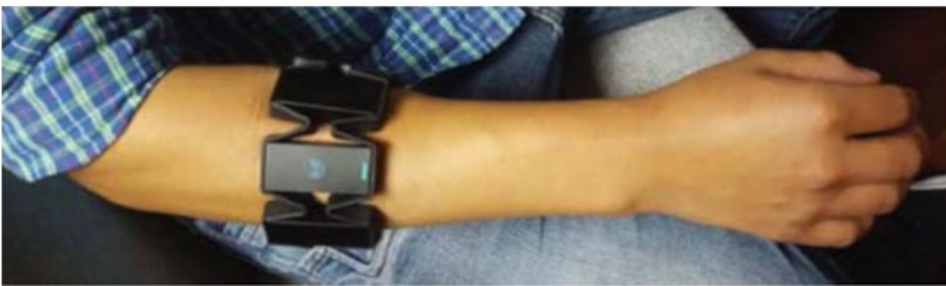
Figure 1 Location of MYO Armband on the Forearm Chung and Benalcázar (2019)
