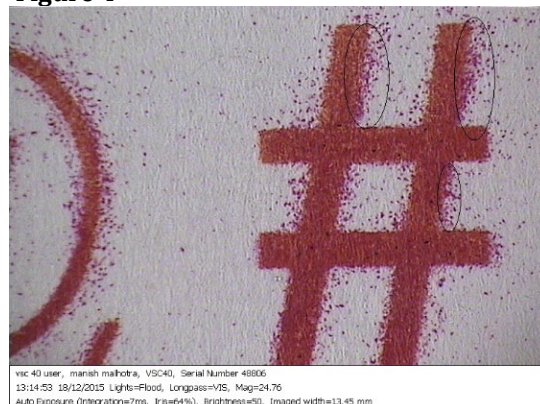
Figure 4 Intense Blooming Effect seen in Brother-DCP J140W
